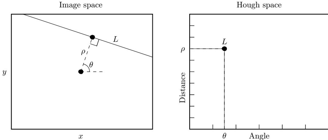
Figure 3: Line  $L$  in the image space maps to a point in the Hough space.
