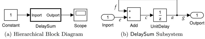
Fig. 3: Simulink model of a counter with step 1.
