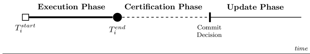
Figure 3.10: Important events and phases in the processing of a transaction in HAcid. Events are represented as nodes and phases are represented as lines.
