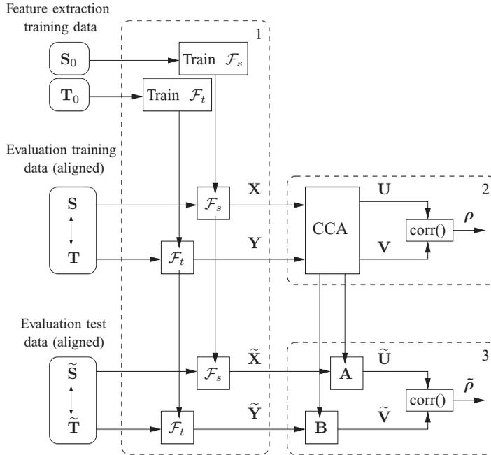
Fig. 2. Diagram of the evaluation setup. (1) The feature extraction method  $\mathcal{F}$  is trained on monolingual corpora and then applied to transform the evaluation data sets into vectorial form. (2) CCA is trained on the evaluation training data to find the canonical variates  $U$  and  $V$  and the respective projection matrices  $A$  and  $B$ . (3) The evaluation test data are then projected into the same space, and finally the test set correlations  $\tilde{\rho}$  are computed.
