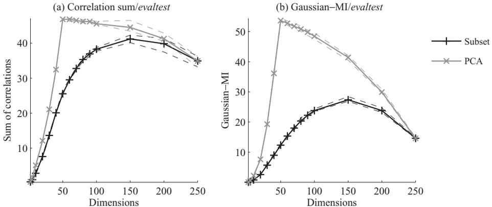
Fig. 6. Evaluation test set results for data with 50 intrinsic dimensions: (a) Correlation sum, and (b) Gaussian–MI score. In subset, a random subset of  $D$  dimensions of  $\mathbf{X}$  and  $\mathbf{Y}$  are selected. In PCA, the  $D$  first principal components are applied. Medians are drawn with solid lines and the first and third quartiles with dashed lines.
