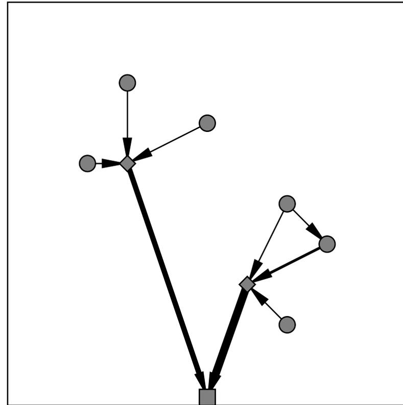
● Sensor node    ◆ Relay node    ■ Sink node
