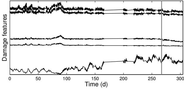
**Fig. 1.** The identified damage features and mean of the standardized bridge deck temperature measurements (lowest curve) for the Z24 Bridge.
