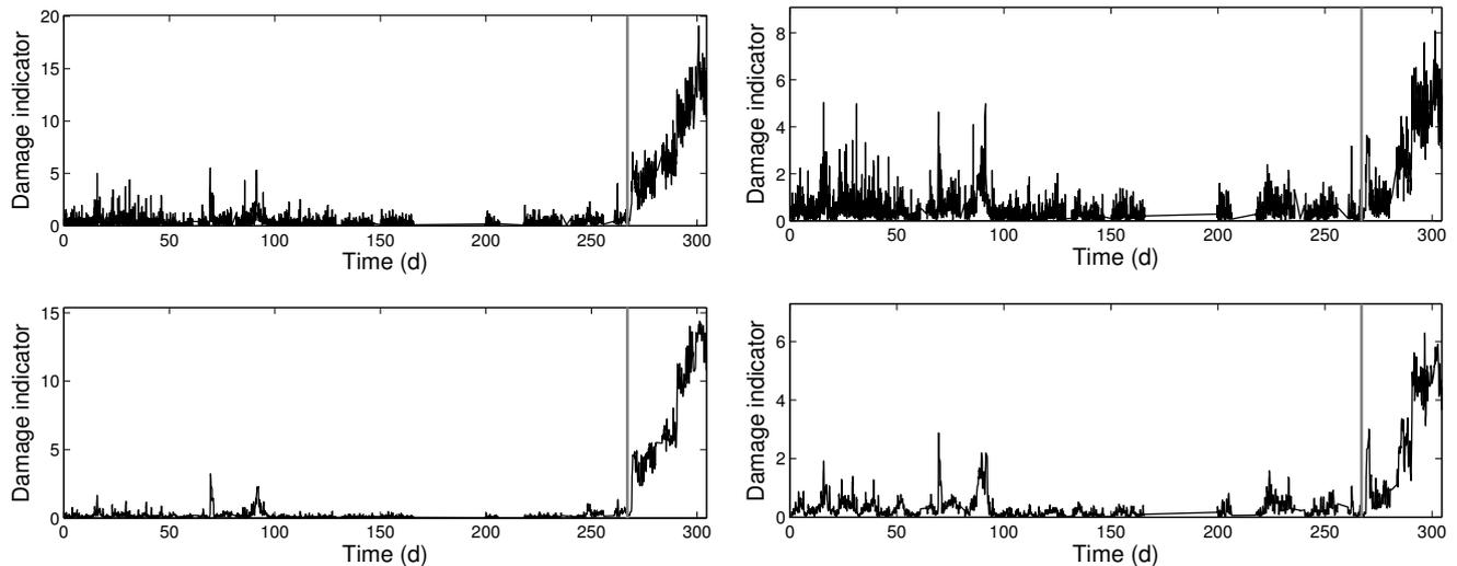
**Fig. 3.** Left: the damage indicator  $d(t)$  by NFA, right: the damage indicator  $d(t)$  by VBPCA. Above: the damage indicator without taking average. Below: moving average of the damage indicator over 5 samples.
