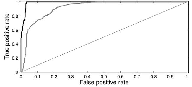
**Fig. 4.** The ROC curve for the NFA and the VBPCA as a function of the threshold.
