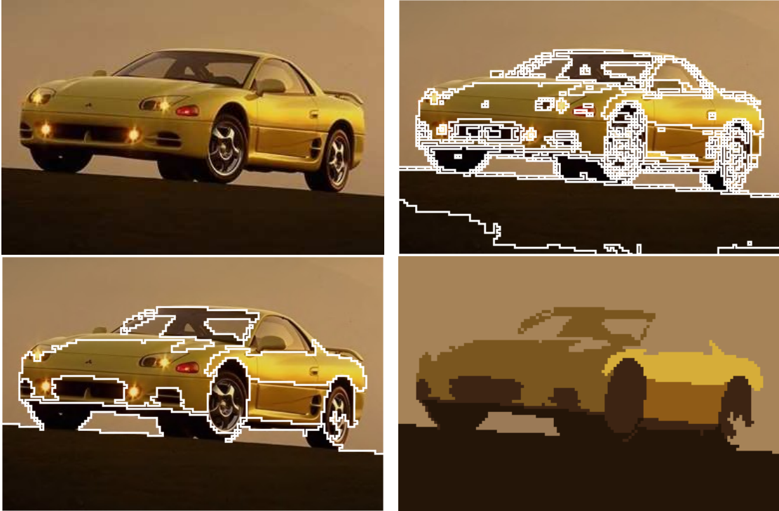
Figure 4.1: An image of a car (top left) with k -means segmentation (top right) and k -means combined with region merging (bottom left). The final segmentation is visualised (bottom right) by colouring each segment with its average colour.
