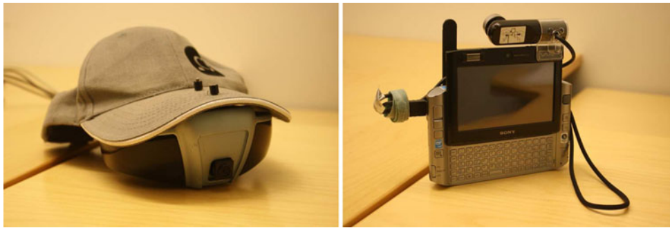
Fig. 4 The display devices. On the left, the head-mounted display (HMD), a wearable near-to-eye display with integrated gaze tracker. On the right, the ultra-mobile PC (UMPC), a handheld computer with virtual see-through display
