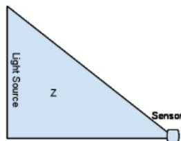
$$p(y_{j,t} | \mathbf{x}_t) = \begin{cases} 1 - \text{FPR} & \text{if } \mathbf{x}_t \in Z_j \text{ and } y_{j,t} = 1 \\ \text{FPR} & \text{if } \mathbf{x}_t \notin Z_j \text{ and } y_{j,t} = 1 \\ 1 - \text{FNR} & \text{if } \mathbf{x}_t \notin Z_j \text{ and } y_{j,t} = 0 \\ \text{FNR} & \text{if } \mathbf{x}_t \in Z_j \text{ and } y_{j,t} = 0 \end{cases}$$
