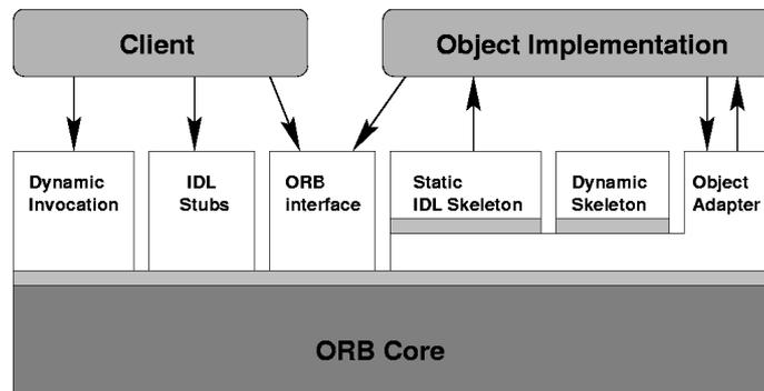
Figure 2. Common Object Request Broker Architecture
