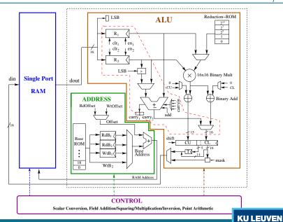
We synthesized the design (coprocessor, not RAM) for UMC 130 nm CMOS with Synopsys Design Compiler
